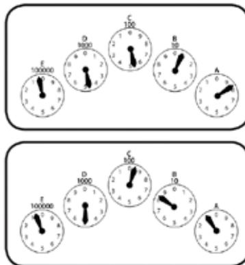
D in the lower diagram, look at the previous dial (C) to the right. If the hand on dial C hasn't passed '0' the number '5' has not actually been reached on dial D and the reading on this dial is the next lower number (4). The reading is therefore 04981.
